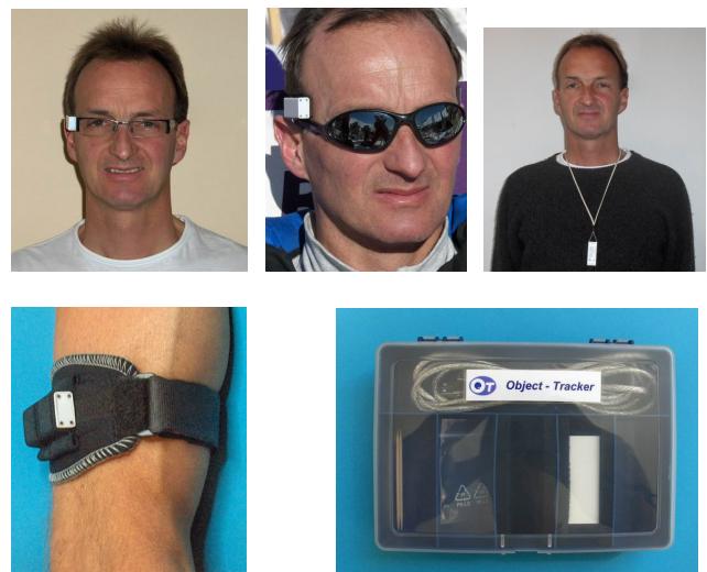
Figure 7: Subjects wearing a data logger attached to eyeglass (left), headset (center), neckband (bottom), and armband (bottom). Transport box with accessories (bottom)
